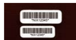
Polyester B423 Top: Pre-reflow Bottom: Post-reflow; Shrunk
