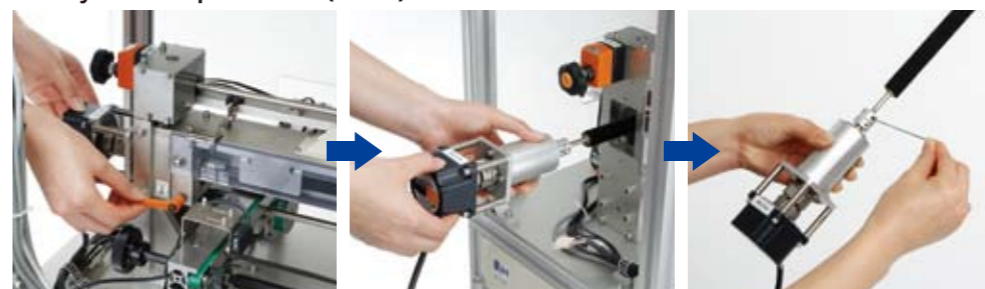
①Releasing lock-lever ②Pulling out brush unit ③Removing brush
